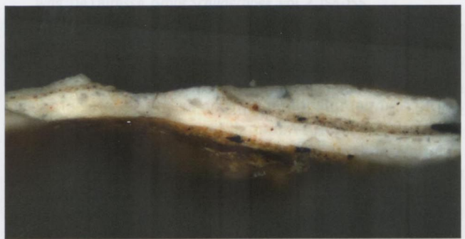
Fig. 8. Cross section taken from one of the arrows (in Concord Trampling Two Enemies , fig. 1A) that was covered with the paint used for the sky.
